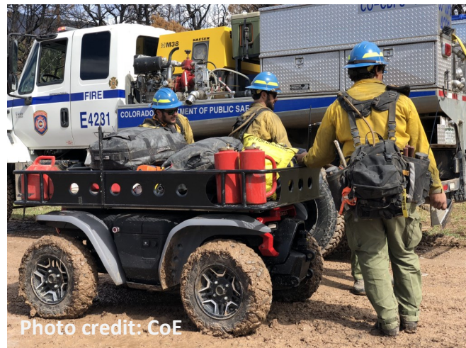
Figure 9— DFPC Montrose Engine Crew loading the Honda Autonomous Work Vehicle for a test run carrying equipment
