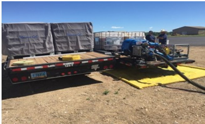
Photo 23: Thermo-Gel FireDos Pumps and Support Trailers at the Craig SEAT Base in 2017 (Photo Credit: CoE)
