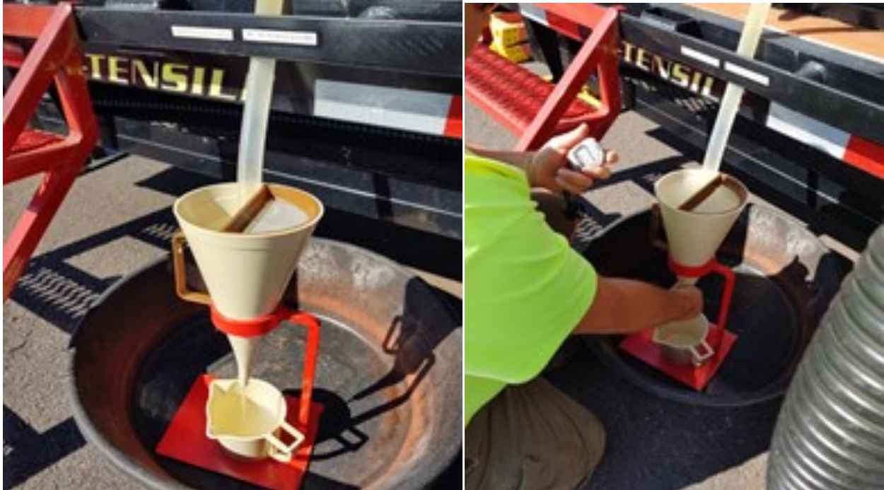
Photos 7 and 8: Marsh Funnel Test for the Viscosity of Firelce 561 (clear) (Photo Credit: CoE)
