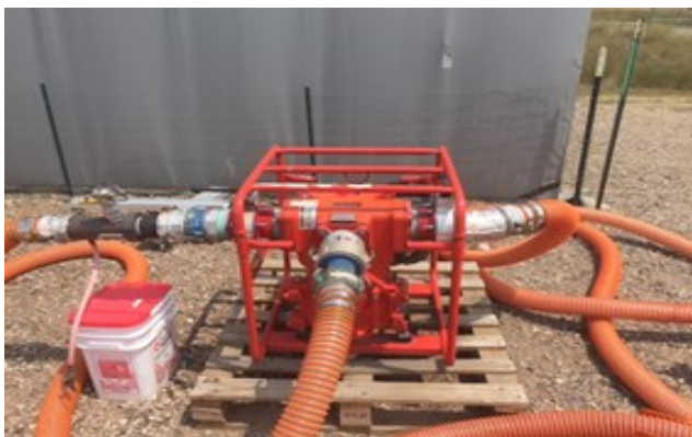
Photos 5 and 6: Pumps for Mixing Firelce at the Fort Collins, Colorado (left) and Roseburg, Oregon (right), SEAT Bases (Photo Credit: CoE)
