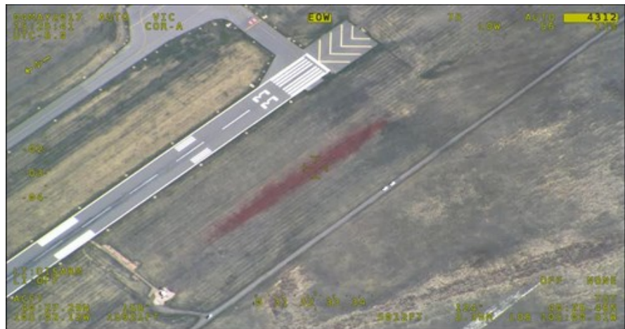
Photo 26: Electro-Optical Color Image of FireIce HVO-F Orange Drop Taken by the MMA in 2017 (Photo Credit: DFPC)
