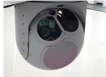
Photo 25: MX-15 Electro-Optical/Infrared Turret (Photo Credit: CoE)
