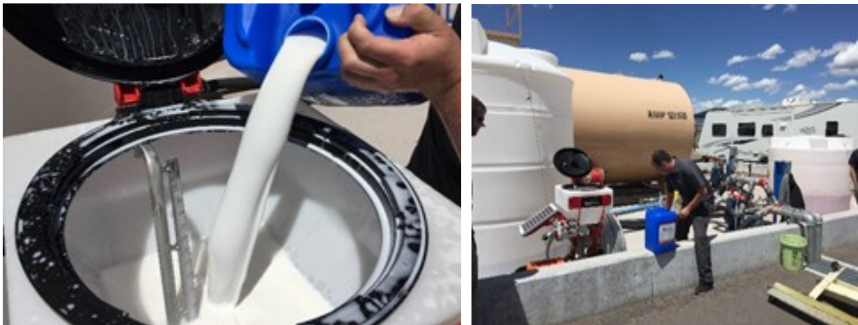
Photos 17 and 18: BlazeTamer 380 Being Poured into the FastFiller Hopper at the Rifle SEAT Base in 2017 (Photo Credit: CoE)
