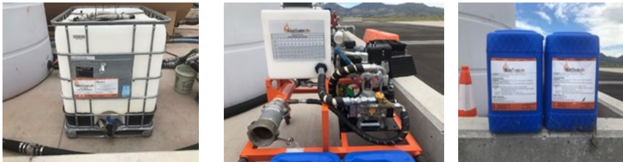
Photos 19, 20, and 21: BlazeTamer 265-Gallon Tote (left), FastFiller 7 (middle), and 5-Gallon Pails (right) (Photo Credit: CoE)
