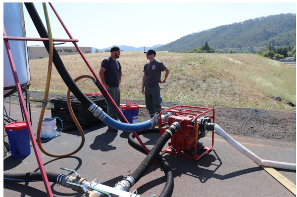
Photos 5 and 6: Pumps for Mixing Firelce at the Fort Collins, Colorado (left) and Roseburg, Oregon (right), SEAT Bases (Photo Credit: CoE)
